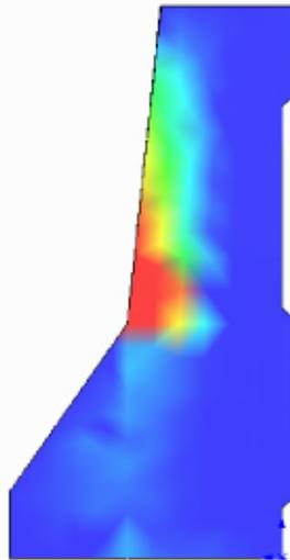
**Figure 16. Partial depth joint cracking predictions.**
