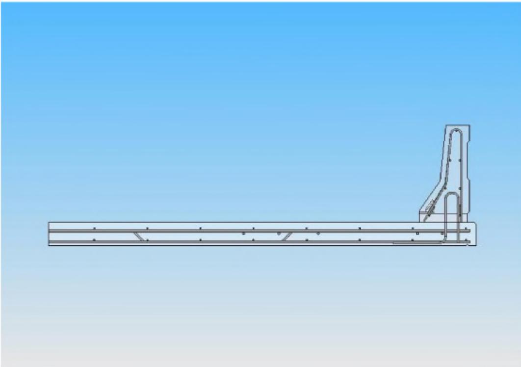
**Figure 8. Side view of the original deck and parapet system.**
