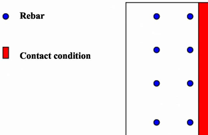
**Figure 11. Connectivity for representative section of parapet bottom.**
