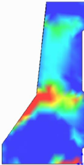
**Figure 14. Cracking prediction for open parapet case.
