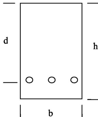
Figure 2. Beam Cross Section
