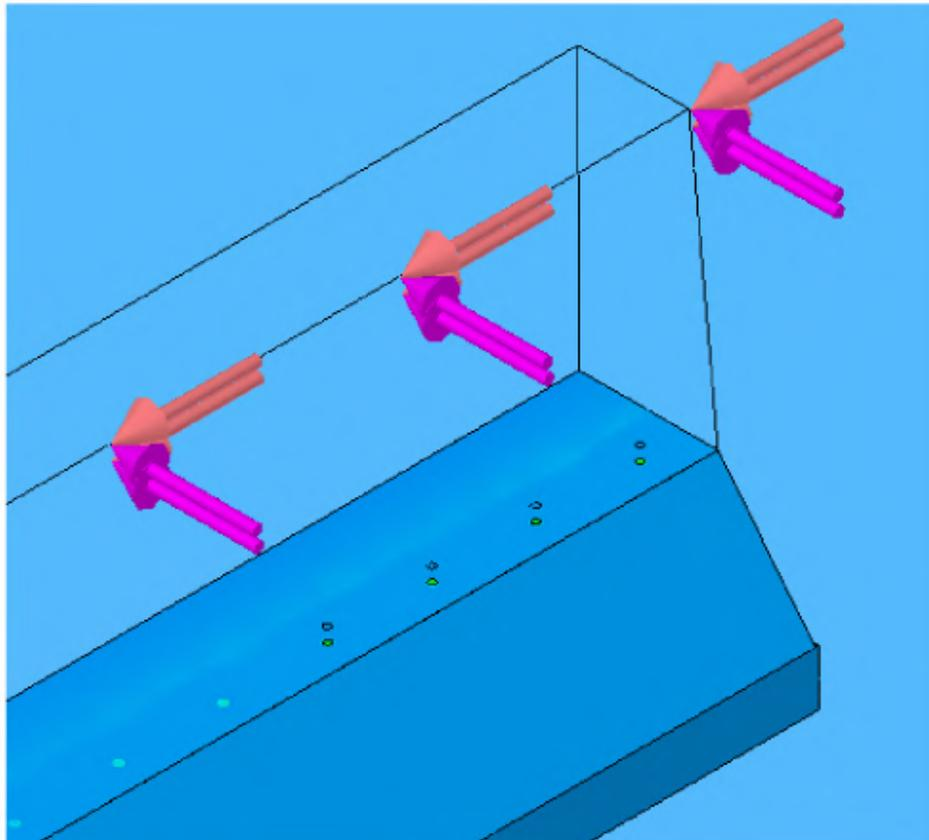
**Figure 9. AASHTO loading designation for proposed parapet. (Top section of parapet shown as transparent to enhance viewing)**
