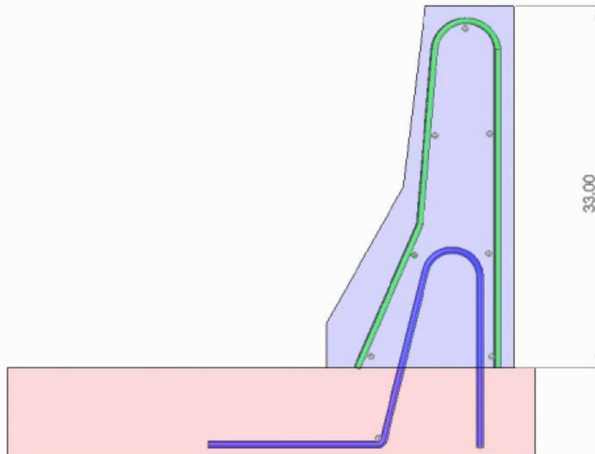
**Figure 12. Modified reinforcement detailing.
