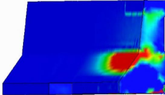
**Figure 13. Cracking predictions for open joint parapet case.
