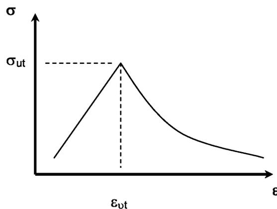
**Figure 1. Post cracked behavior using tension stiffening model.**
